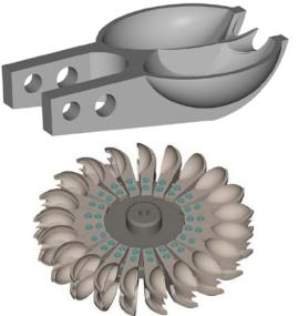
Fig.11 Bucket and Runner for Designed Pelton Turbine
