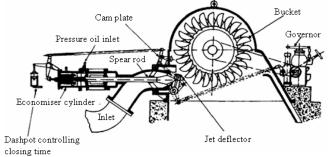
Fig. 1 Main Components of Pelton Turbine [1]
