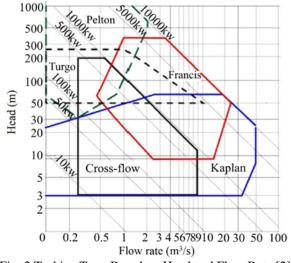
Fig. 2 Turbine Type Based on Head and Flow Rate [2]
