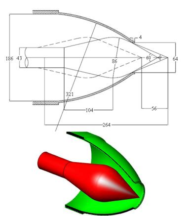
Fig.12 Nozzle with Needle for Designed Pelton Turbine
