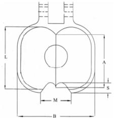
Fig. 5 Bucket Dimensions for Pelton Turbine [6]
