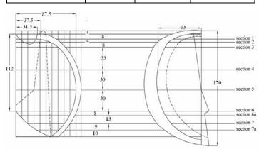
Fig.9 Front View and Side View of Bucket
