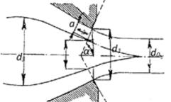
Fig. 7 Cross Section of Nozzle at the Position of the Needle [6]
