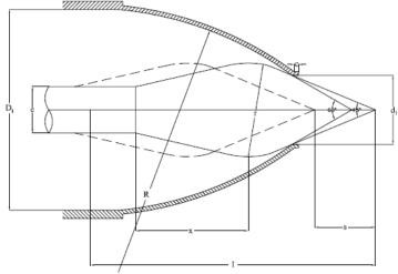
Fig. 8 Profile of Nozzle and Needle [6]
