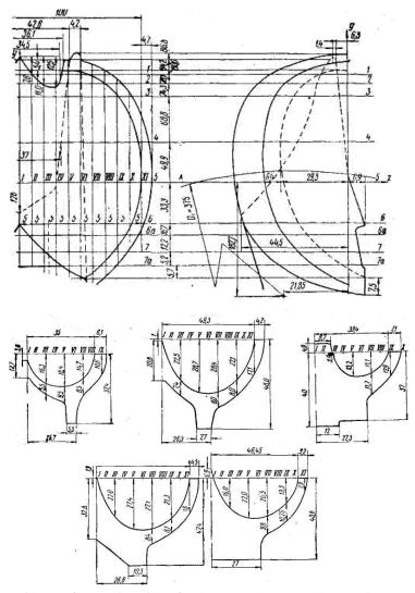
Fig. 6 Referenced Design of a Structure Stream To-461 Bucket Turbine [3]
