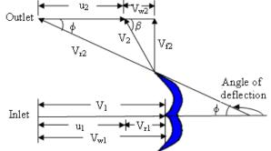
Fig. 3 Inlet and Outlet Velocity Triangles of Pelton Wheel [1] Where,
